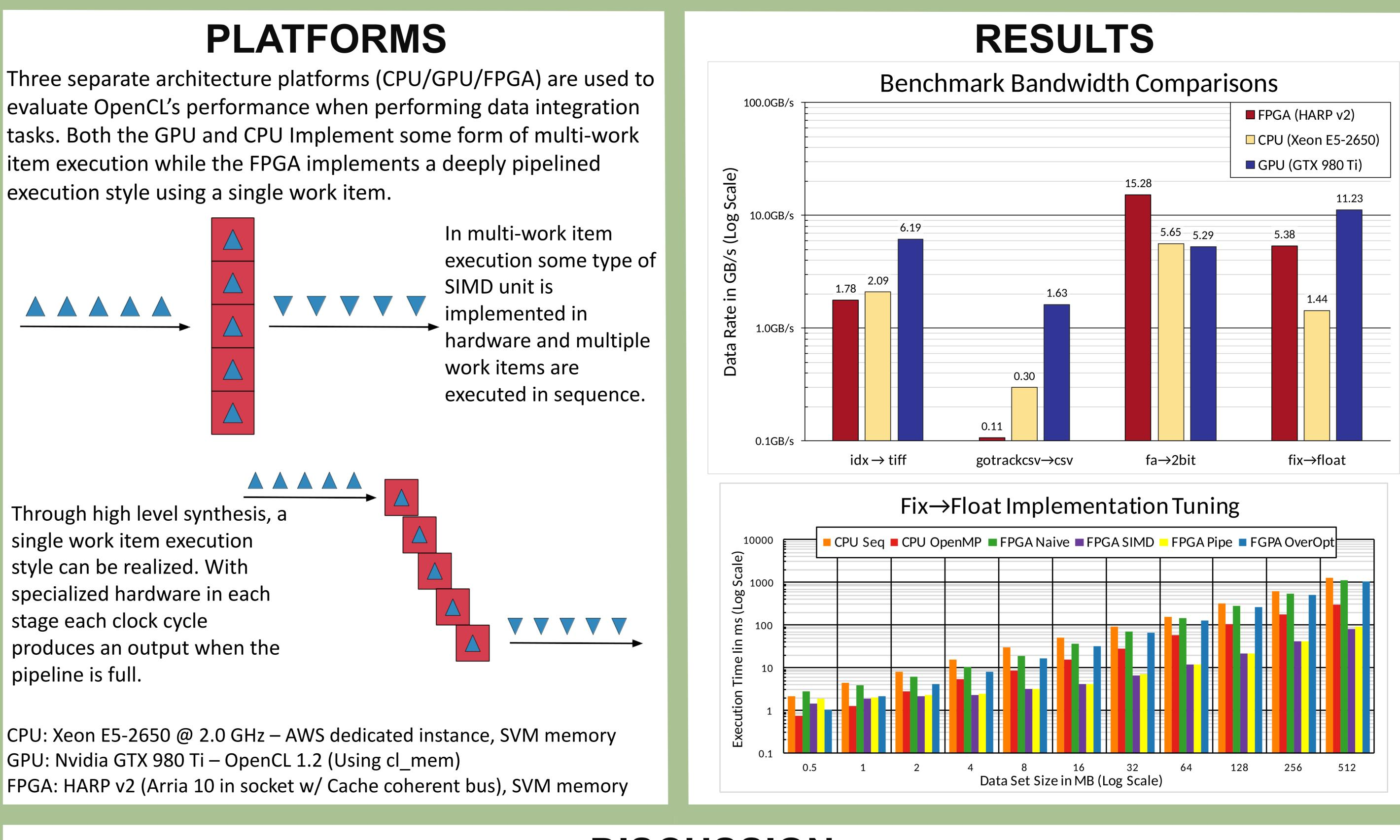
Through high level synthesis, a single work item execution style can be realized. With specialized hardware in each stage each clock cycle produces an output when the pipeline is full.
